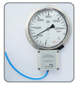
TEST LEVEL BUTTON - This is an override facility and can be operated at any time, if the button is pressed and held, the reading will rise then fall slightly, release button and allow to settle, reading can now be taken.
